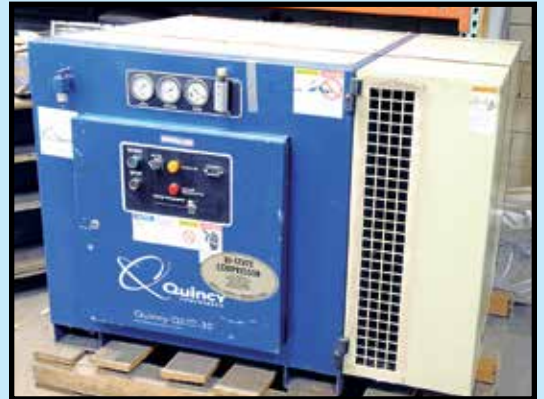
QUINCY 30 HP ROTARY SCREW AIR COMPRESSOR
