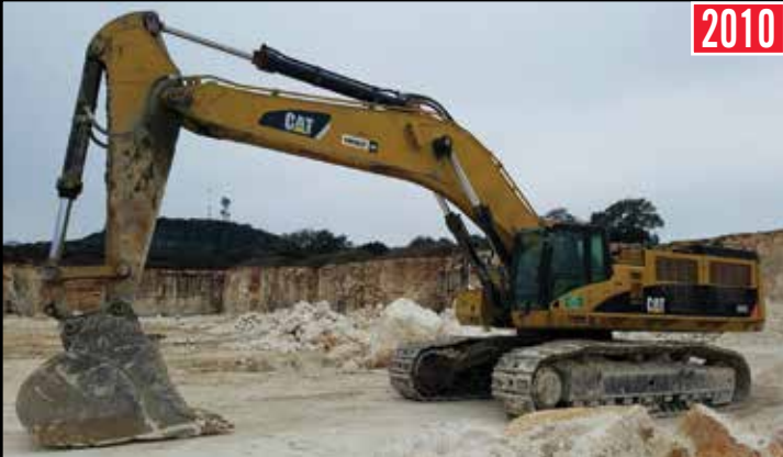
CAT 385CL Hydraulic Excavator
