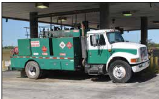
INTERNATIONAL 4900 Fuel & Lube Truck
